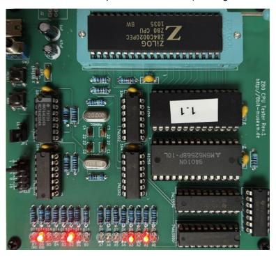
The identified U880 displays 01000100 (Port B). "U" is set, "tttt" is 0100.
