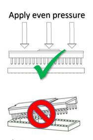
Do NOT bend vLA128 or insert at an angle
