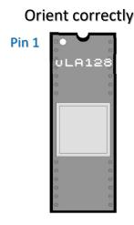
6. Apply even pressure across the vLA128 top surface and press into the ULA socket.
