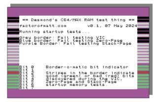
The border stripes show address bits (A0-A15, top-to-bottom) and data bits (D0-D7, top to bottom). A black address bit is 1, light grey is 0. A green data bit indicates a good bit, red indicates bad. Here we see that data bit 2 was detected as bad and that the most recent memory location found to be bad was \$01B3.
